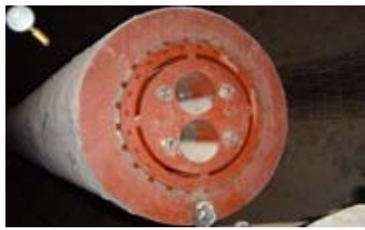
A burner for petcoke, solid wastes (two channels), liquid wastes/heavy fuel oil ( http://www.dynamis-ma.com/ ).
