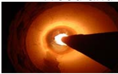
A burner for petcoke, solid wastes (two channels), liquid wastes/heavy fuel oil ( http://www.dynamis-ma.com/ ).
