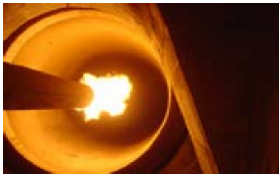
Burner for petcoke, solid wastes, natural gas / diesel oil lance. ( http://www.dynamis-ma.com/ )
