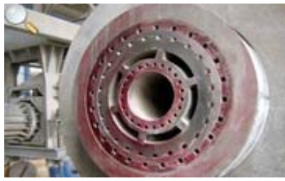
Burner for petcoke, solid wastes, natural gas / diesel oil lance. ( http://www.dynamis-ma.com/ )
